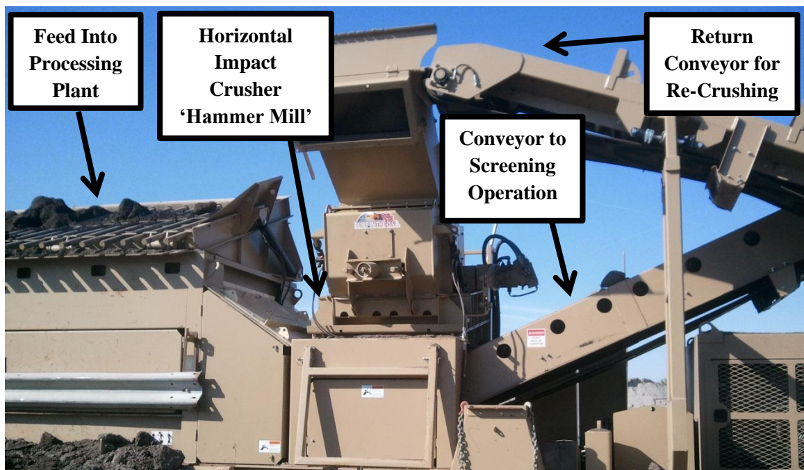
Figure 2-3: RAP Processing Equipment - Hammer Mill Crusher
